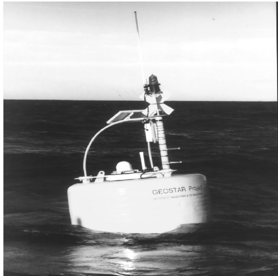
Fig. 4. The Near Real Time Communication System buoy
