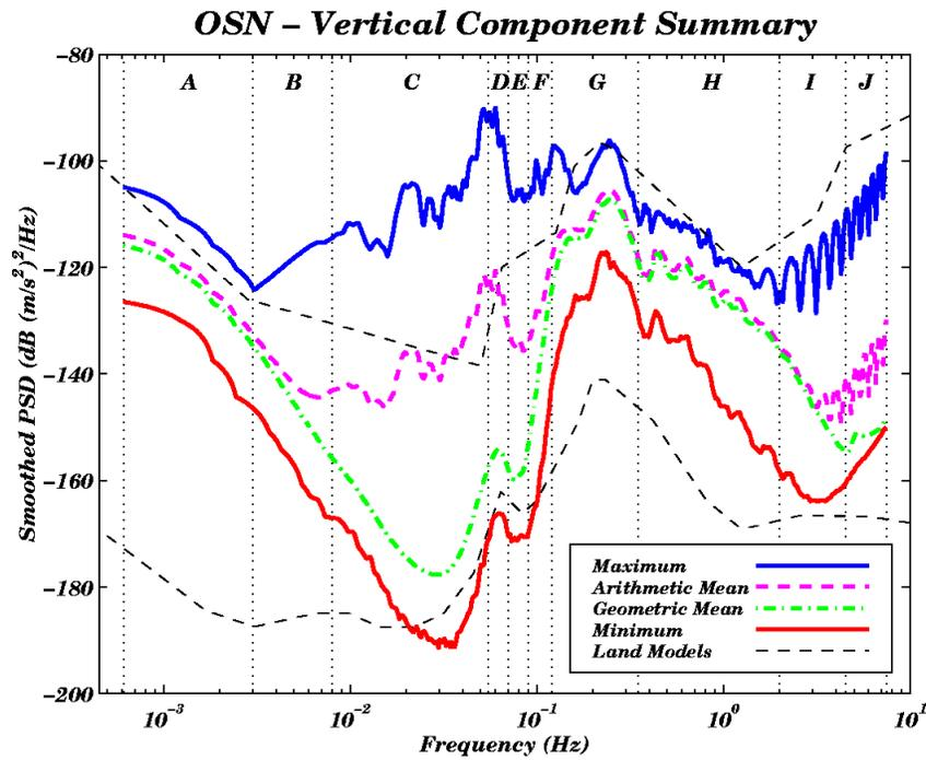
Figure 3: Summary of OSN power spectral densities which were computed every 1.82hrs for the whole data set.
