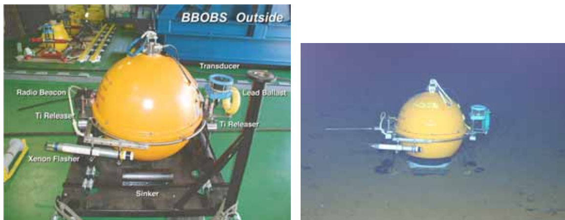
Fig. 2.2.5. Photographs of the BBOBS on the ship deck (left) and upon the seafloor
